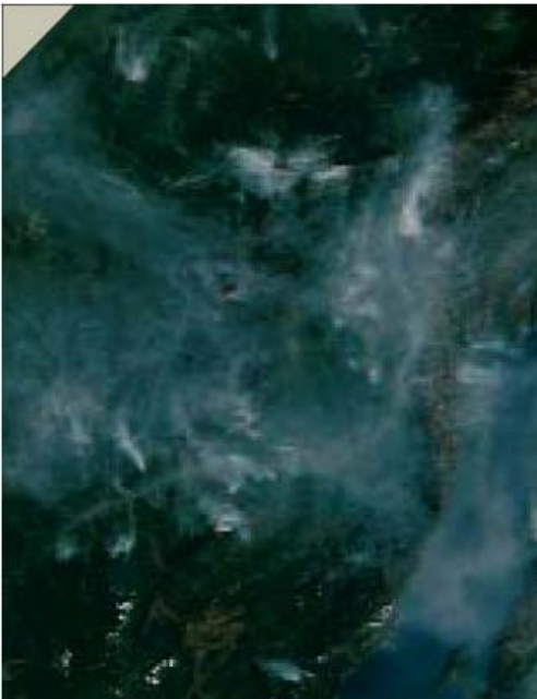
Fig. 5. Low resolution images of MODIS 36-channel spectral radiometer of Terra/Aqua satellites are largely used in Russia to resolve tasks related to daily near real-time monitoring. The most common practical application of MODIS data is the on-line monitoring of forest and grass fires. The image illustrates the Baikal area fires in August 2005. Resolution 250 m. Red spots – areas, delineated with automatic algorithms of fire detection.
