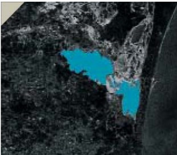
Fig. 7. Middle resolution radar data of RADARSAT-1 satellite are successfully used in Russia in ice reconnaissance, forestry and hydrology. The Terek river delta image was acquired on May 25, 2005 from RADARSAT-1 per the request of the Water Resources Federal Agency of the Russian Ministry of Natural Resources to access the damage of the flooding and to work out an emergency response plan with respect to the catastrophic breakthrough of the protection embankment in the Terek river estuary. Flooded areas are shown in color (image processed by State Oceanographic Institute specialist)
