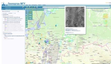
In 2010, the MSU Geoportal was created - the geo-information complex, which includes hardware ("UniScan-24" complex, data processing terminals, terminals to work with the geoportal, computer room, server of MSU's geoportal); software (software products designed to work with Earth remote sensing data), as well as a databases of satellite images and maps, which are regularly replenished with new imaging materials.
